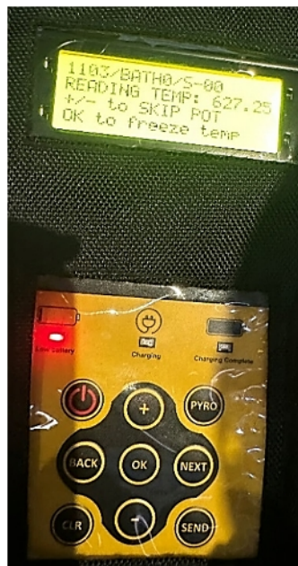
Figure 8. Bath temperature measurement.
