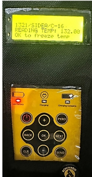
Figure 7. Collector bar temperature measurement.
