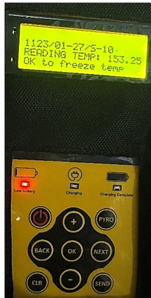
Figure 5. Side shell temperature measurement.
